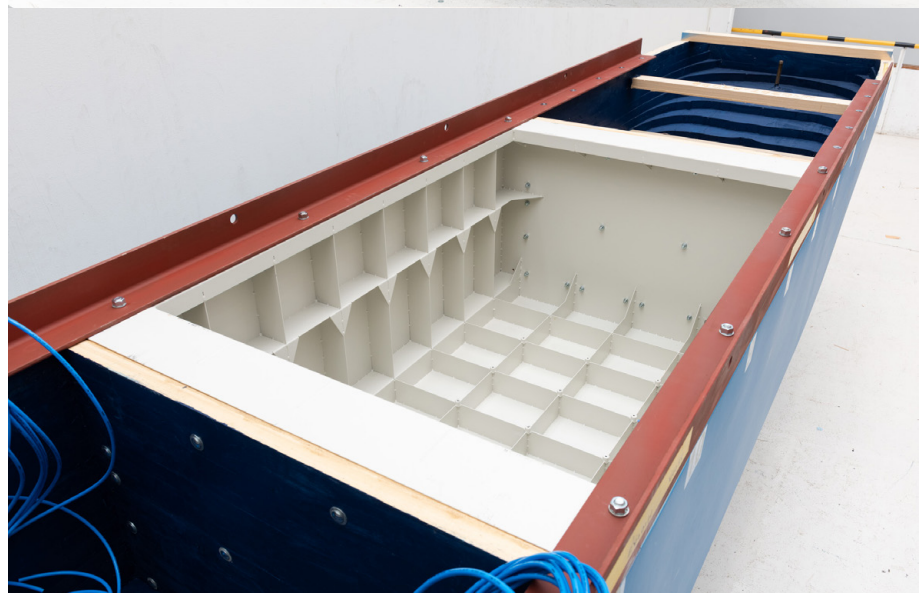
Above: View of the 7.8 metre long ship model hull with steel midsection. See image on the next page for a snapshot of air bubble layer under the ship model hull, injected through porous hoses.
