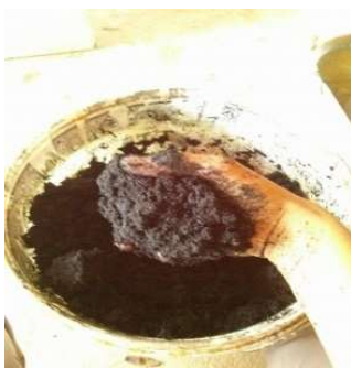
Figure 57: Moist biochar to reach approximately 80% of moisture
