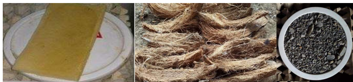
Figure 48: Materials used to provide water: sponge (left), coconut rip (middle), trays with rubble (right)
